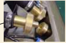
A detachable part of the cable (YSI-25D Ver.2)
